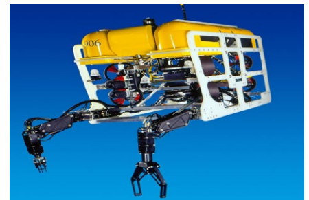
The ROV frame is made from extremely rugged polypropylene chassis with a stainless steel lift frame.
