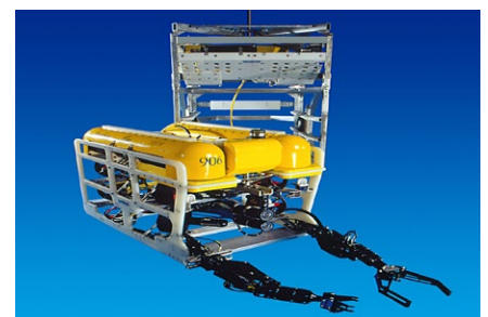
The 2 electronics pods provide most of the Panther Plus buoyancy. Additional buoyancy is provided by shaped syntactic foam blocks.
