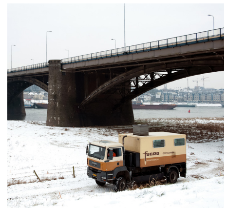
TarGOST®-CPT investigation with a track truck during winter.
